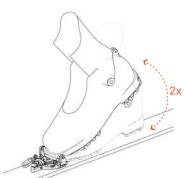
MOVE TO ENSURE THE PINS FIT PROPERLY INTO THE SHOE
